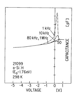
Fig.3.4. Set of four C-V characteristics at 298 K corresponding to different measuring frequencies for undoped a-Si:H/p c-Si ( $N_A$ =1.0x10 $^{16}$  cm $^{-3}$ ) heterojunction.
