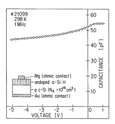
Fig.3.3. C-V characteristics of undoped a-Si:H/p c-Si heterojunction.
