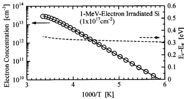
FIG. 1. Temperature dependence of the majority-carrier concentration for the  $1 \times 10^{17} \text{ cm}^{-2}$  electron irradiated  $p$ -type Si. The open circles represent the experimental  $n(T)$ , and the solid line represents  $n(T)$  interpolated by the spline function. The broken line represents the temperature dependence of the Fermi level.
