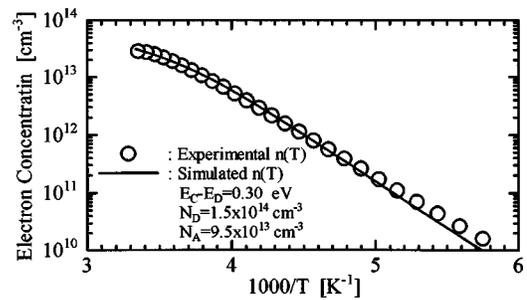
FIG. 3. Temperature dependence of the electron concentration. The open circles represent the experimental  $n(T)$  and the solid line represents the  $n(T)$  simulated with the obtained values.
