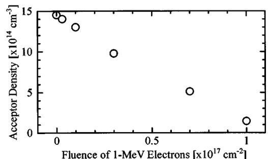
FIG. 4. Dependence of  $N_B$  determined by FTIR on the fluence of 1 MeV electrons.
