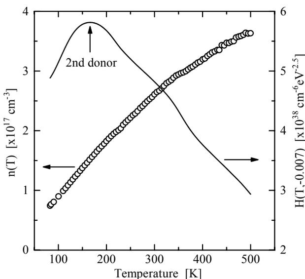
Fig. 1  $n(T)$  and  $H(T, -0.007)$  for 8- $\mu\text{m}$ -thick 3C-SiC
