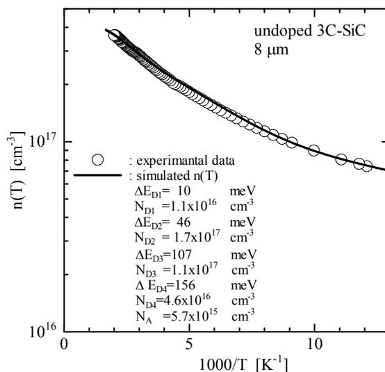
Fig. 3 Experimental and simulated  $n(T)$
