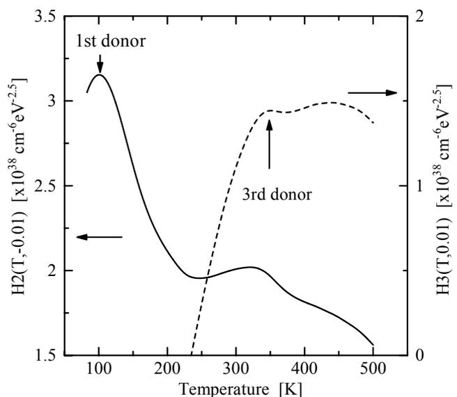
Fig. 2  $H2(T, -0.01)$  and  $H3(T, 0.01)$  for 8- $\mu\text{m}$ -thick 3C-SiC
