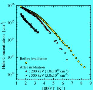
Although the fluence of 200 keV electrons is higher, the p(T) decreases less than due to 500 keV electron irradiation.
