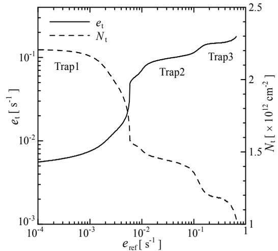
Fig. 6. The  $e_{\text{ref}}$  dependence of  $e_{ti}$  and  $N_{ti}$  determined from the maximum of the DCTS signal.
