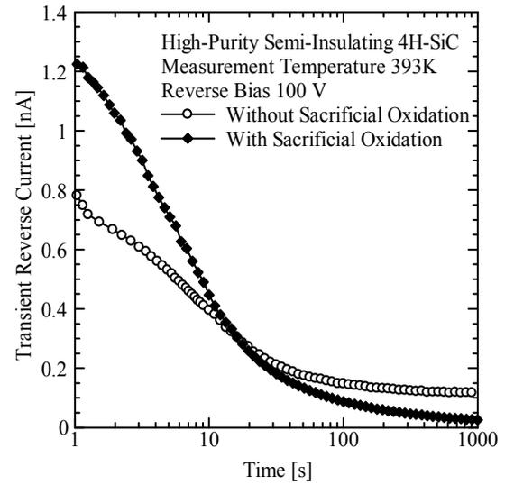
Fig. 2. Transient reverse current for devices fabricated on surfaces with and without sacrificial oxidation.
