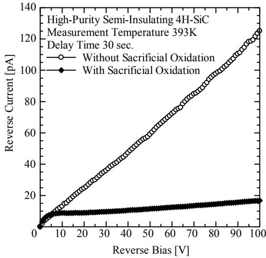
Fig. 1.  $I-V$  characteristics for devices fabricated on surfaces with and without sacrificial oxidation.
