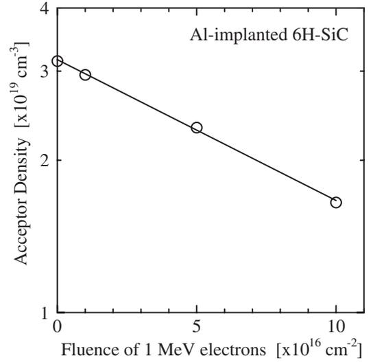
Fig. 2. Fluence dependence of corrected acceptor density.
