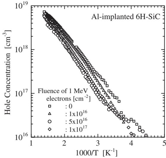
Fig. 1. Temperature dependence of hole concentration for Al-implanted 6H-SiC unirradiated or irradiated by 1 MeV electrons at three fluences.
