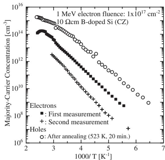
Fig. 1. Temperature dependence of electron concentrations in first and second measurements, and hole concentration after annealing. Each measurement was carried out from low  $T$  to high  $T$ .
