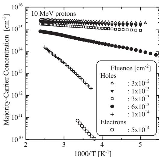
Fig. 2. Fluence dependence of hole concentration in Si irradiated by 10 MeV protons.
