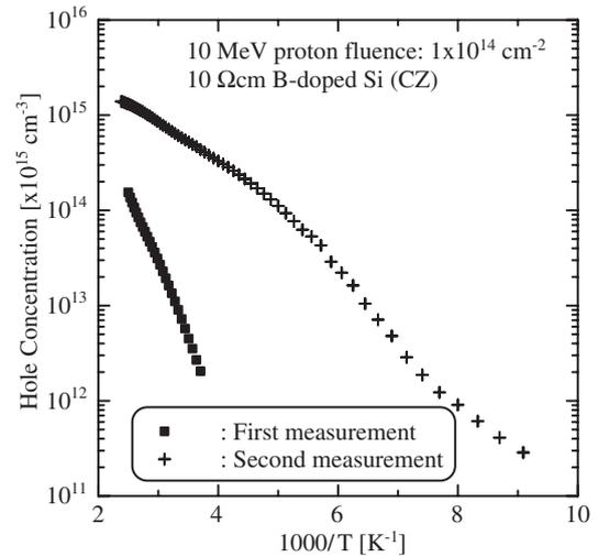
Fig. 3. Temperature dependence of hole concentrations in Si irradiated by 10 MeV protons with  $1 \times 10^{14}$  cm<sup>-2</sup> fluence in first and second measurements. Each measurement was conducted from low  $T$  to high  $T$ .
