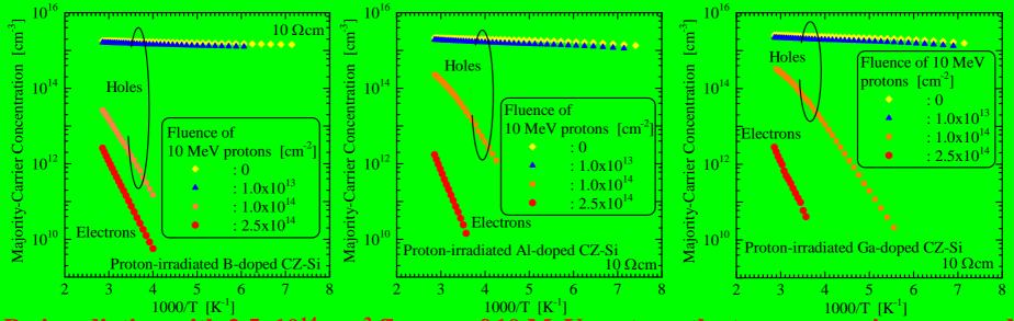
By irradiation with 2.5x10<sup>14</sup> cm<sup>-2</sup> fluence of 10 MeV protons, the type conversion occurred in the 10  $\Omega$  cm CZ-Si with any acceptor species (B, Al, Ga).
